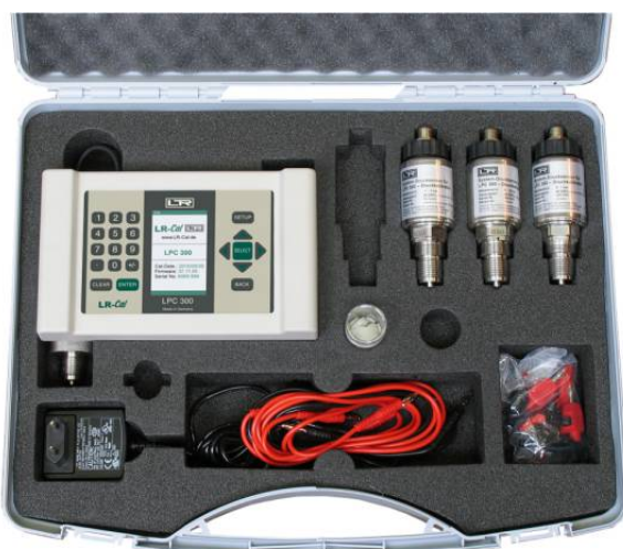
Image (left): LR-Cal LPC 300 with 4 reference sensors LR-Cal LPC-S in optional transit case.
