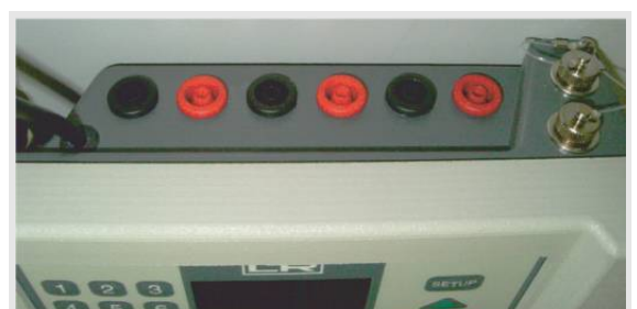
Image: Electrical ports at the LR-Cal LPC 300
