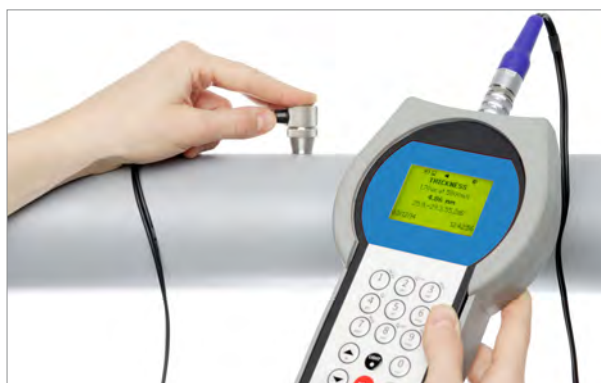
Wall thickness gauge NT with USCX200 in use
